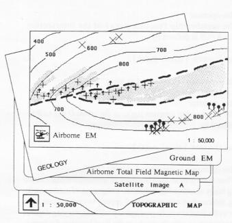
Fig. 1. Schematic diagram of spatial information layers.
