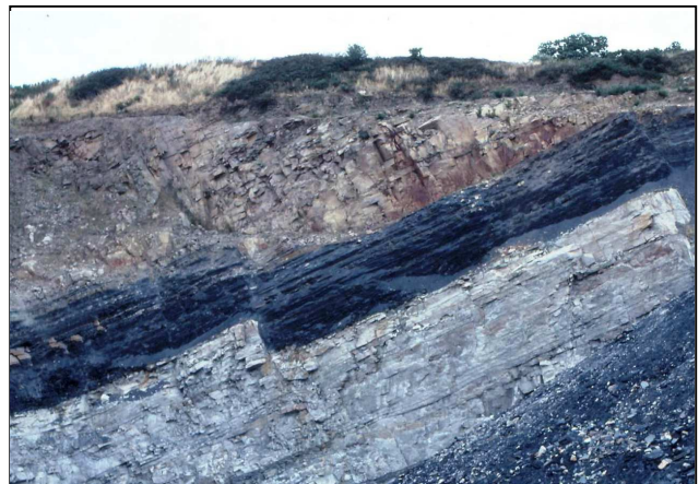
A normal strike fault dipping in the opposite direction to the dip of the bedding – showing how beds can be repeated. A Carboniferous coal seam in an opencast coal mine. Skelmersdale, Lancashire. UK.
